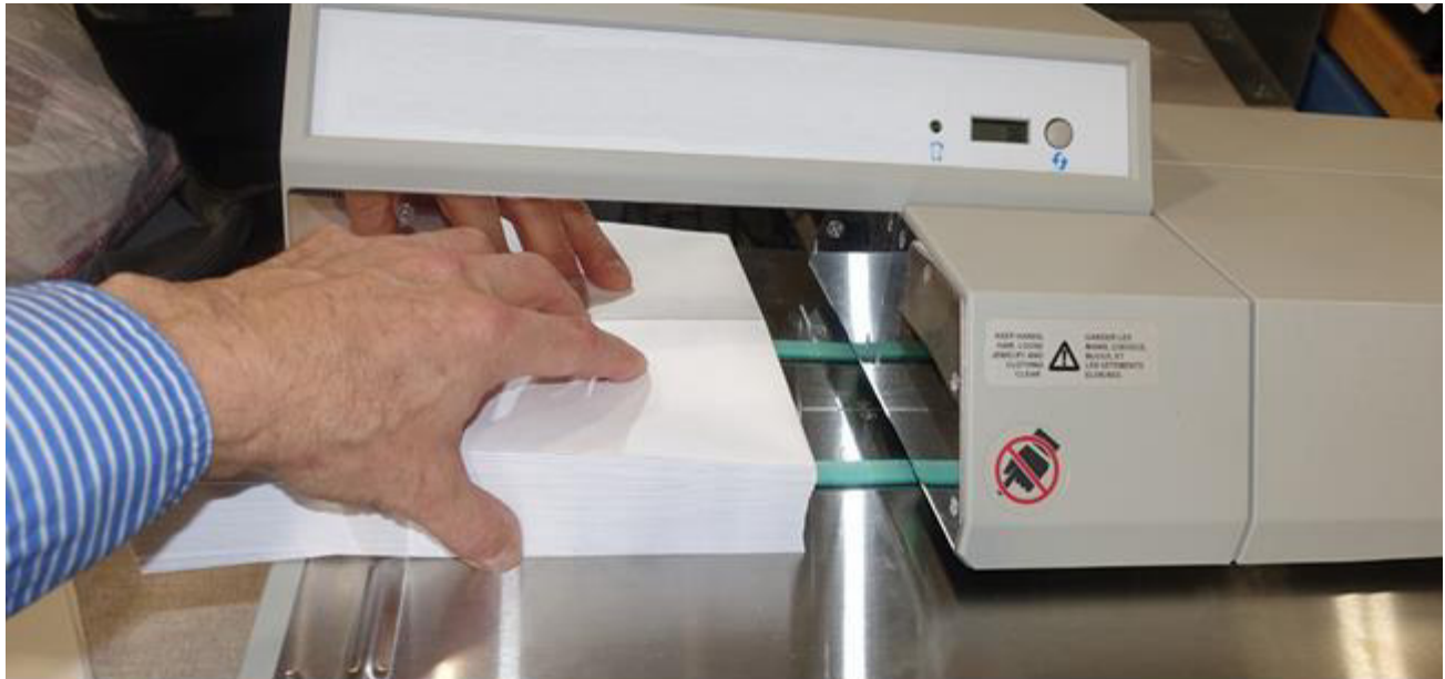
Figure 4-6: Loading the Envelope Feed Hopper
