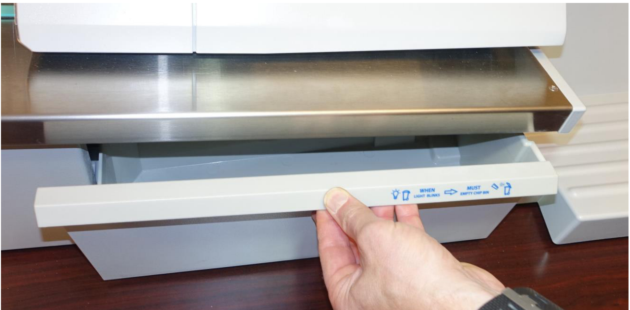
Figure 2-8: Bin tray removal interlock triggering
