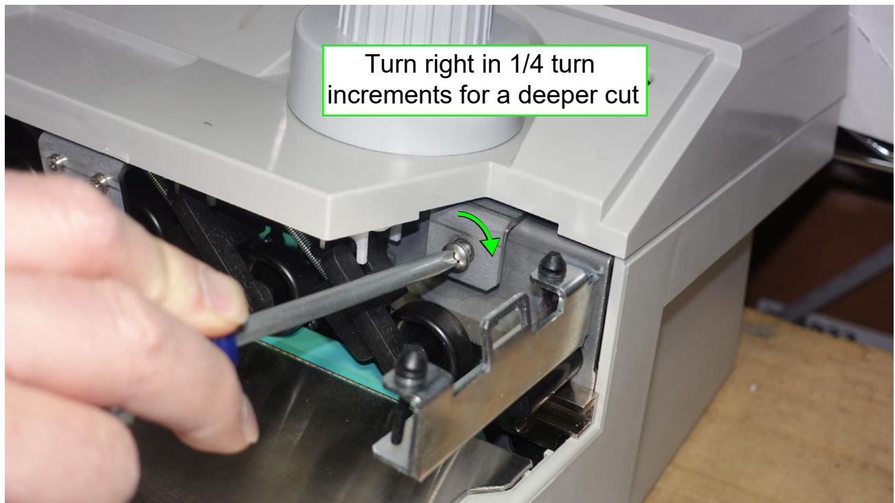
Figure 4-18: Adjusting the cutter depth
