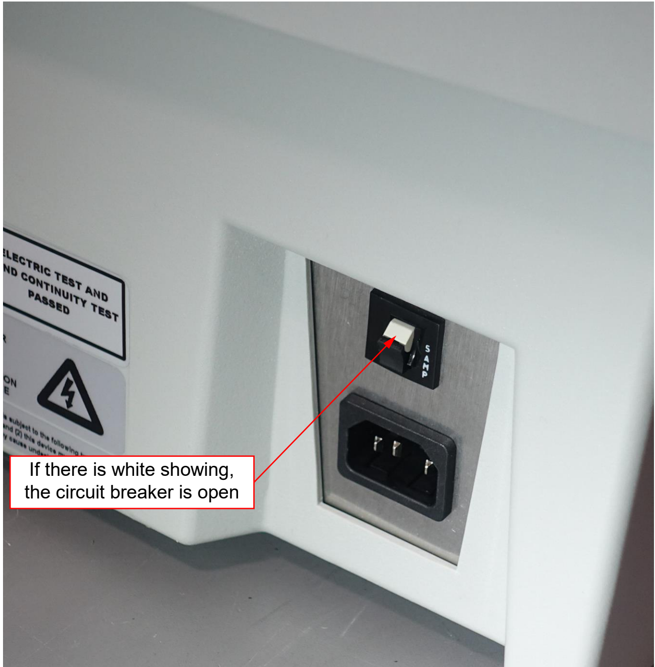
Figure 4-19: Open circuit breaker
