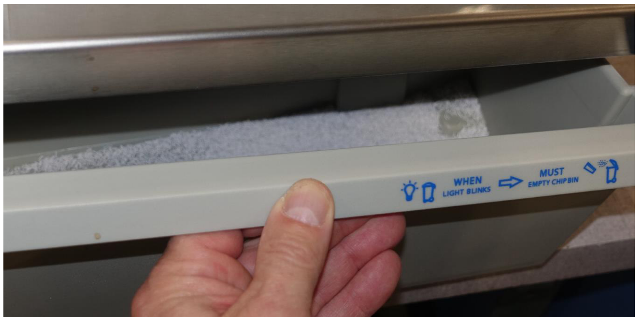
Figure 4-3: Opening the Chip Bin tray
