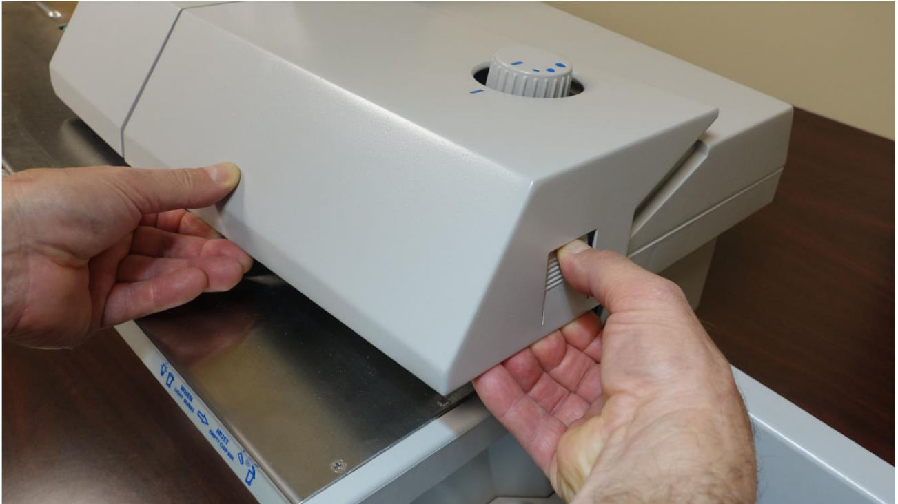
Figure 2-7: Top cover removal interlock triggering
